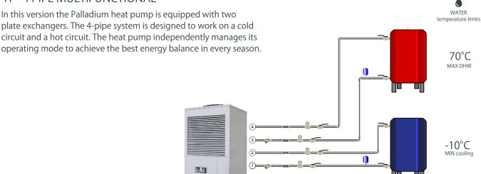
(1/2) Users input/output (3/4) Recovery input/output
